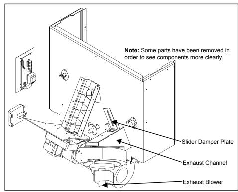
Figure 22: Slider / Damper
